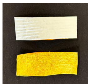
Figure 1. Membranes' pieces showing the outer PHBV/microwires layer (top) and the inner Cs/PEO/CUR one (down).
