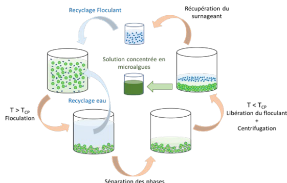
Figure 1 Representation of the complete targeted microalgae culture cycle, flocculation, concentration of the solution in microalgae and release/recycling of flocculant.
