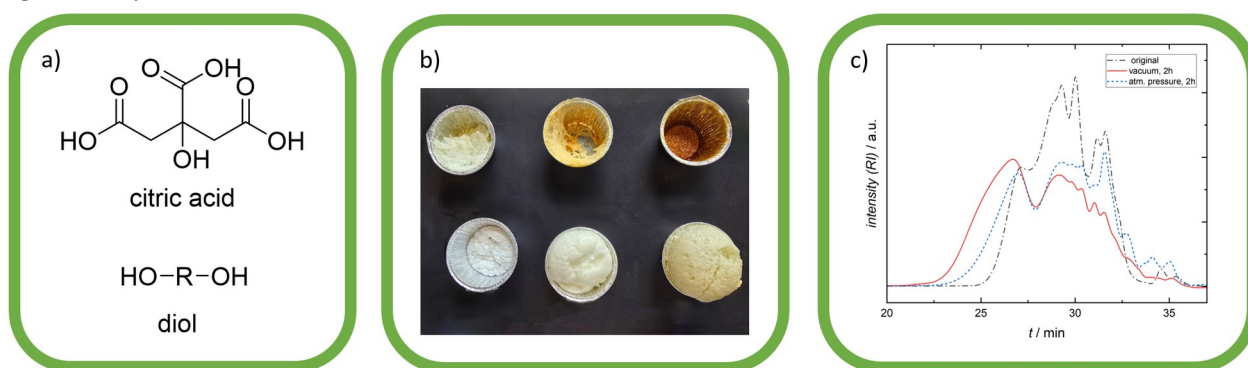
Figure 1: a) Monomers used for polyester synthesis. b) Products of crosslinking condition screenings. c) GPC allows good comparison of polyester crosslinking conditions before obtaining insoluble networks.
