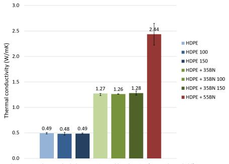
Thermal conductivity values measured perpendicularly to injection molding direction for samples with different content of the BN filler: 0, 35, and 55 wt.%. Results are shown for reference pristine samples and samples after testing shape memory effect. Bars with standard deviation are indicated for each type of specimen.
