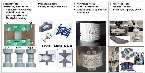
Fig. 1: Overview of the specimen configurations and test methods
