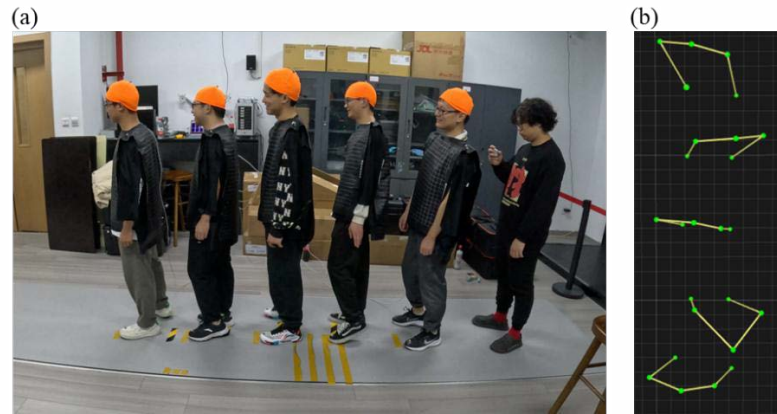
Figure 1: (a) side-view video recording and (b) Top-down view from Qualisys motion capture data, with trajectory points of the head, shoulders, and feet connected for clear differentiation, demonstrating the condition of asynchronous swaying at a step frequency of 45 bpm.
