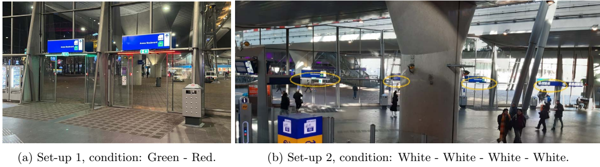
Figure 1: The experiment uses two different set-ups: (a) lights installed above two exit doors, and (b) lights installed above four adjacent exit doors, highlighted with yellow contours.
