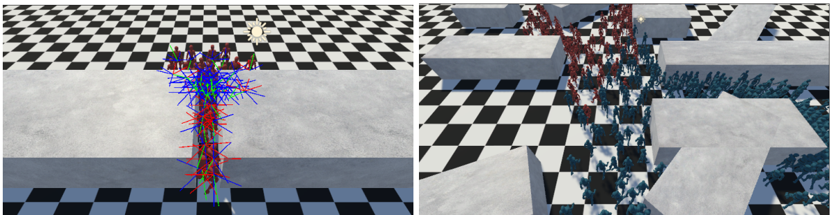
Figure 2: Left - example visualization of bottleneck simulation based on real-world data, right - theoretical scenario. The red line is the repulsion vector from walls, the blue line is the repulsion vector from other agents, and the green line is the direction of motion (the resultant of all forces acting on the agent).
