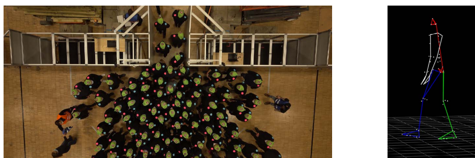
Figure 1: Experimental setup and motion capture data. (Left) Top camera view from bottleneck experiment, and (Right) corresponding motion capture data from one participant, illustrating the detailed movement patterns recorded.
