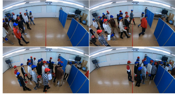
Figure 2. Images taken during the experiment (blue caps for typical walkers and red for slow walkers).
