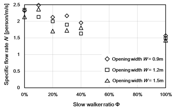
Figure 3. Relationships between the specific flow rate N and the slow walker ratio \Phi .
