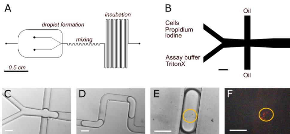
**Figure 1.** Microfluidic chip for cell lysis. Scheme of the chip (A). Scheme of the chip inputs (B). Micrographs of: (C) cell encapsulation; (D) mixing of droplet content; (E) lysed cells (bright-field mode); (F) lysed cells (epifluorescence mode). Scale bar: 100  $\mu$ m.
